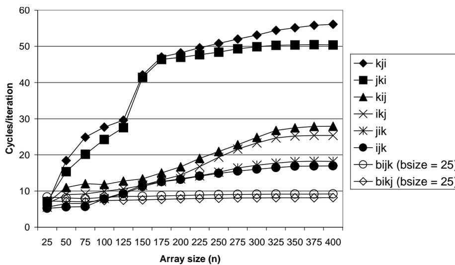
Figure 3: **Pentium III Xeon blocked matrix multiply performance.** Legend: *bijk* and *bikj*: two different versions of blocked matrix multiply. The performance of different unblocked versions is shown for reference.
