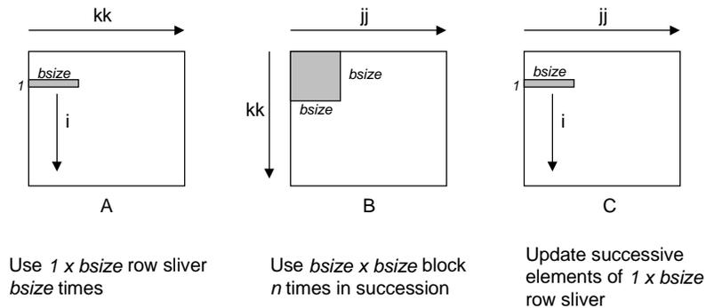
Figure 2: **Graphical interpretation of blocked matrix multiply** The innermost ( $j, k$ ) loop pair multiplies a  $1 \times bsize$  sliver of  $A$  by a  $bsize \times bsize$  block of  $B$  and accumulates into a  $1 \times bsize$  sliver of  $C$ .
